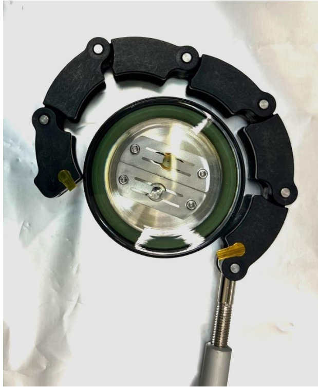
Figure 7: Remove plastic chain clamp from assembly.
