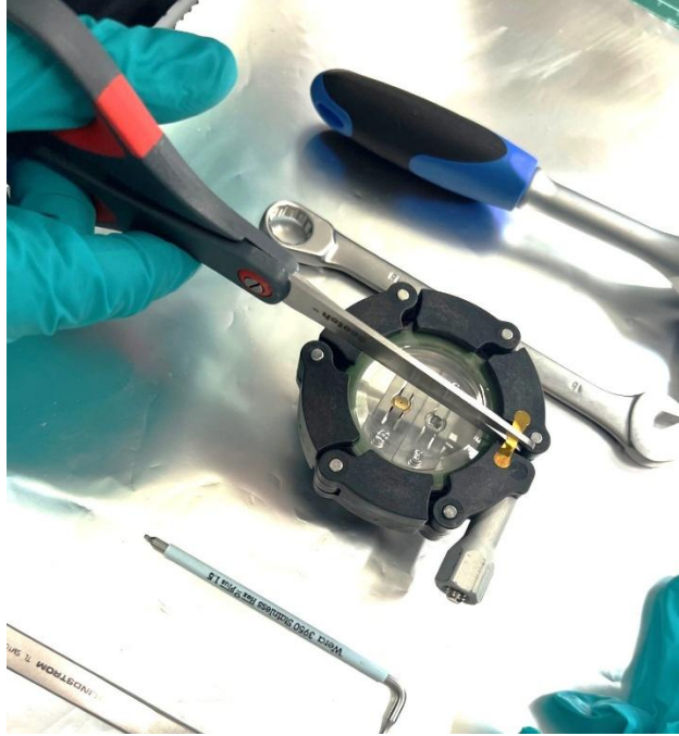
Figure 5: Cut open the securing tab.
