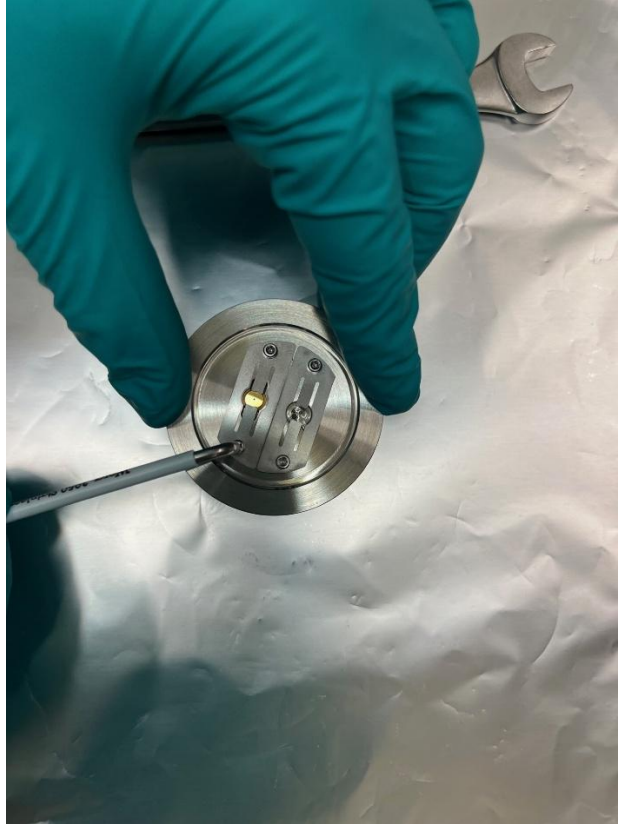
Figure 9: Unscrew hex bolts from metal clamping spring securing the MAS.
