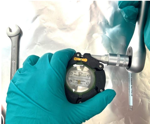
Figure 6: Loosen the thumb nut on the plastic chain clamp using socket wrench.
