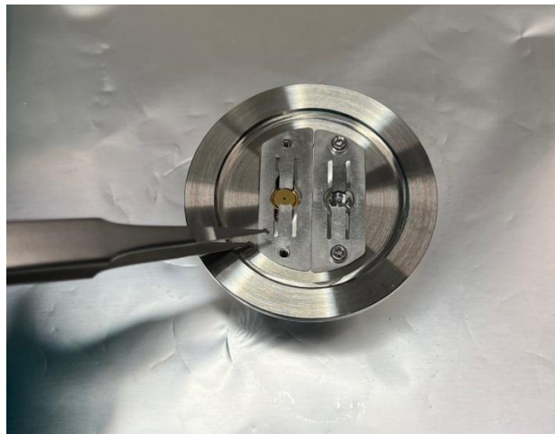
Figure 10: Remove metal clamping spring using tweezers.
